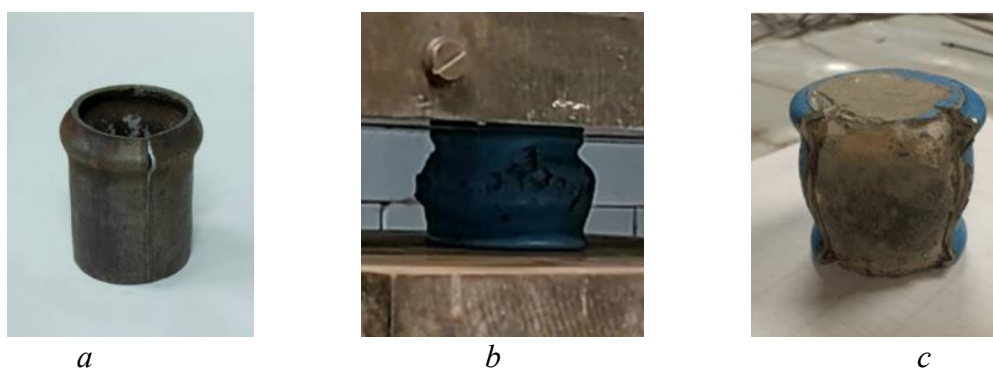
Fig. 3. Steel tube (a) and tube specimens (b) specimen after axial compressive load tests; deformed state of the concrete core after the transition to the plastic phase (c)
