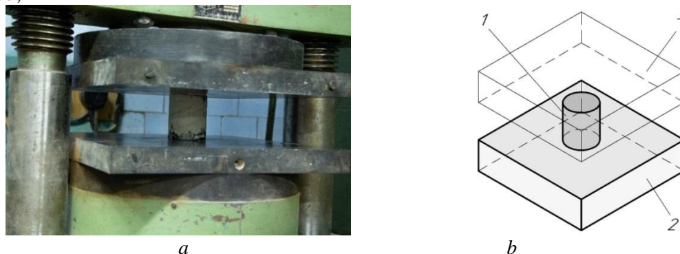
Fig. 3. Testing specimens 100 mm long: a – general view; b – schematic diagram of the experimental setup: 1 – tested specimen; 2 – movable loading plate; 3 – fixed loading plate
