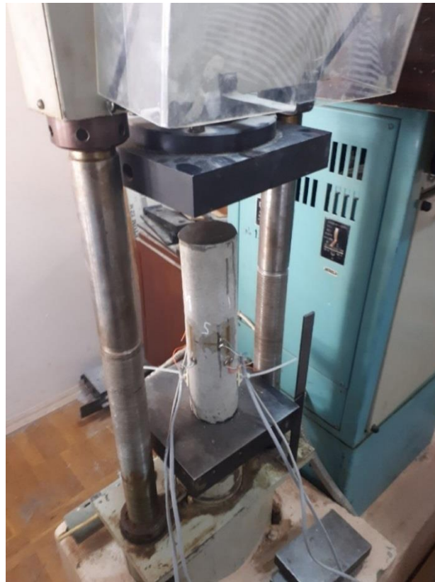
Fig. 5. Installation for tensometric testing of concrete
